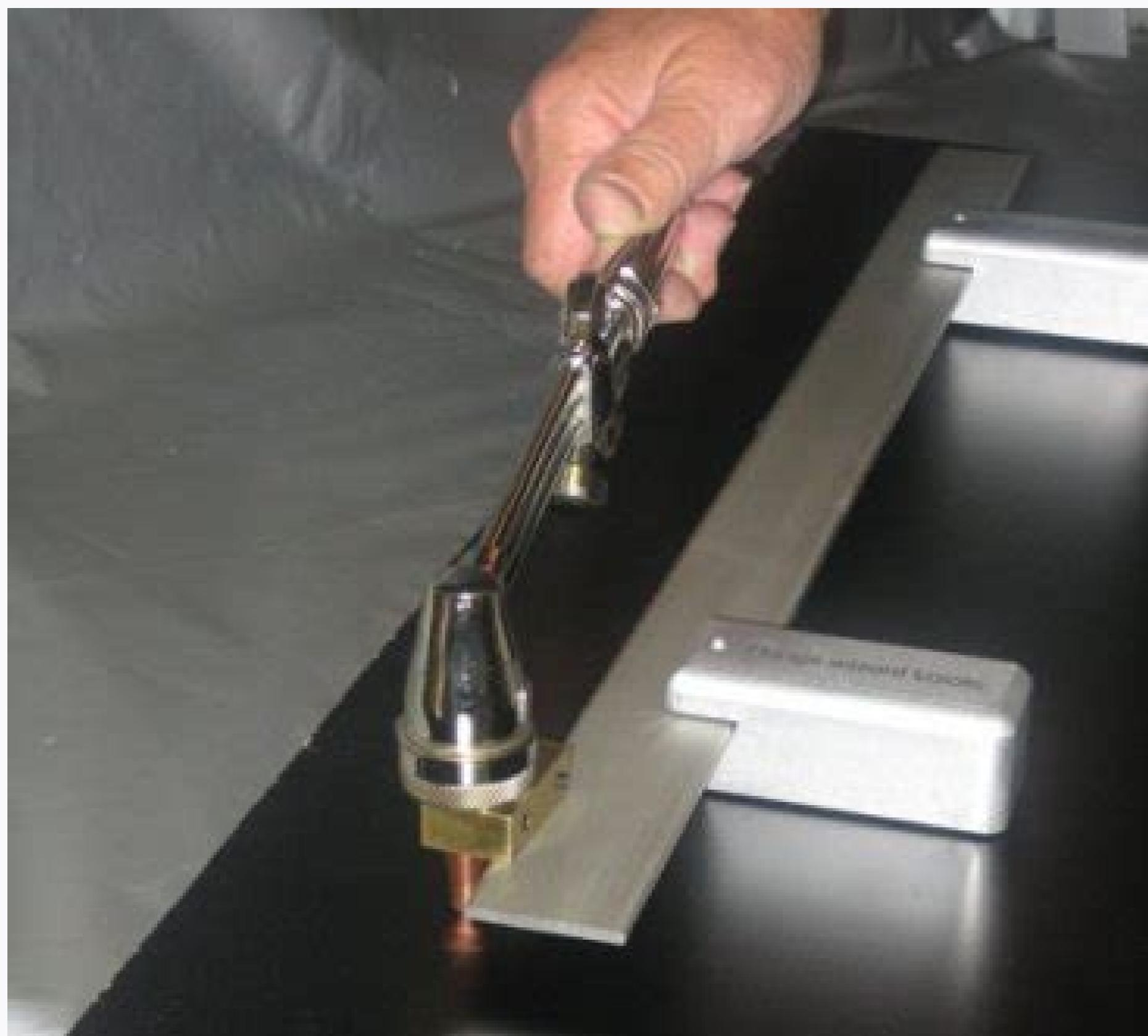
Cnc plasma cutting tips and tricks. Tips and tricks for plasma cutting. Tips for plasma cutting. Plasma cutting magnetic guide strip. Eastwood magnetic plasma cutting guide.
